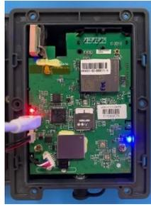
Figure 6: Red and blue LED lights begin to blink once connected
