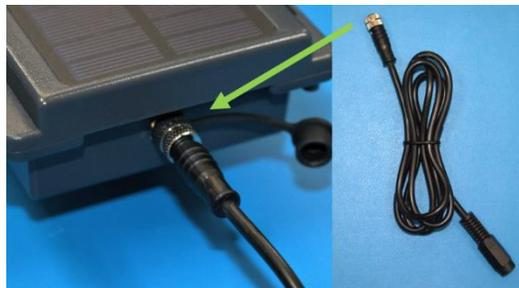
Figure 16: Connecting the power cable
