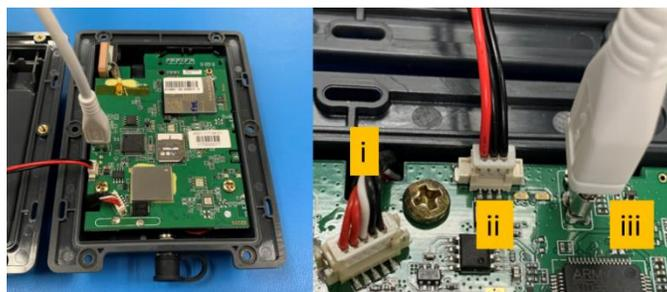
Figure 5: Connecting cables, right image POV is oriented 90 degrees clockwise
